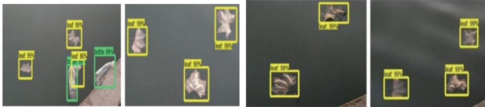
Fig.6 Detection results of floating garbage on the water surface
